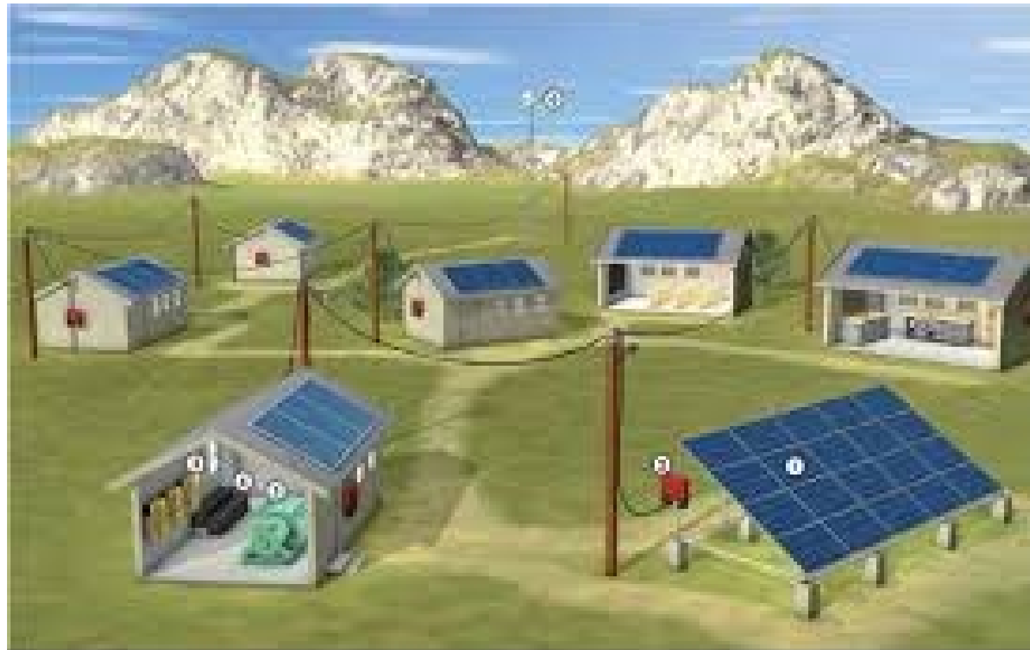
Components: 1 - PV array, 2 - TRANSFORMER, 3 - BATTERY BANK, 4 - Batteries, 5 - Diesel generator, 6 - Wind turbine system
